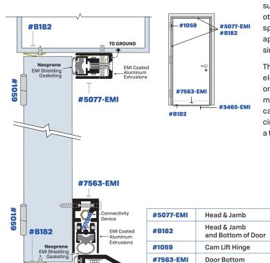
System #6090EMI is one solution available from Legacy for blocking electromagnetic and radio frequency interference in applications such as laboratories, hospitals, brokerage houses, embassies and other facilities using sensitive electronic equipment. We can provide specification assistance for configuring other systems for specific applications. Legacy also offers OEM consultation for developing similar systems.
