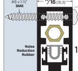
• Self-leveling door seal up to maximum 7/8" drop.
