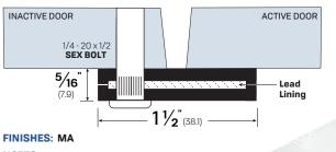
Lead Lined Material for X-Ray protection.
