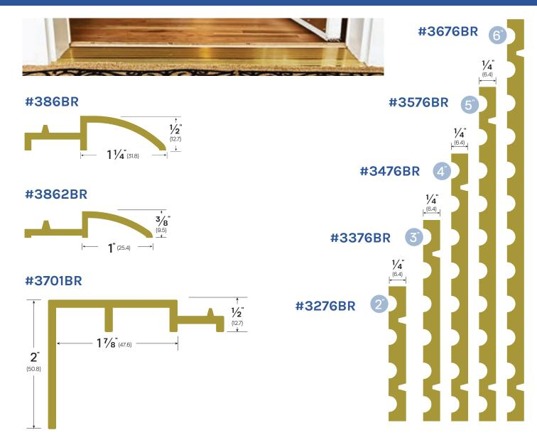
$\textbf{Various Configurations} \quad \textbf{\textcircled{6}} \quad \textbf{Configurations made from adjustable bronze thresholds}.$
